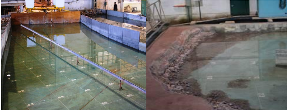
Figure 3.2 - Irregular wave tank, a) General look; b) Bathymetry, Fortes et al., 2007
